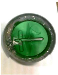
In this attack the skimming device is part of the false overlay bezel. This bezel is attached on top of the legitimate card reader bezel. In addition some form of device or method is also installed to capture the user PIN data.
